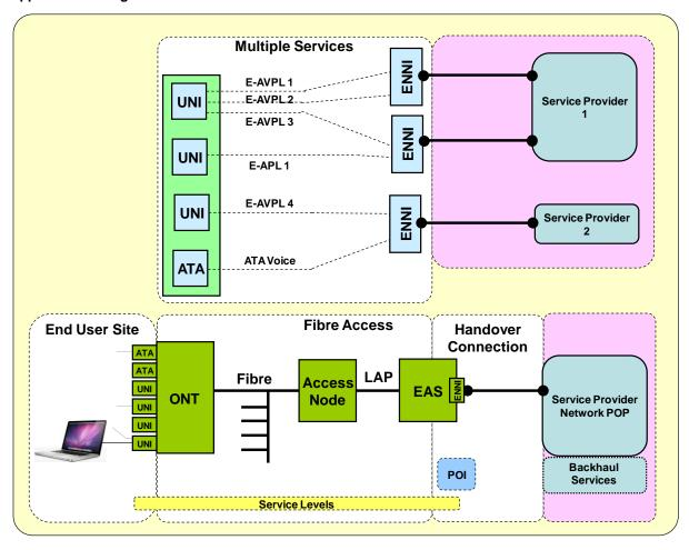
This is a generic diagram showing the standard configuration and Service Demarcation Points. It is not intended to represent every situation or detailed physical architecture. The following points should be noted:
